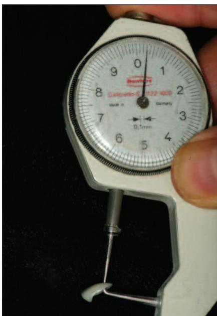
**Figure 16.** Veneer thickness measured an average of 0.3 mm.
